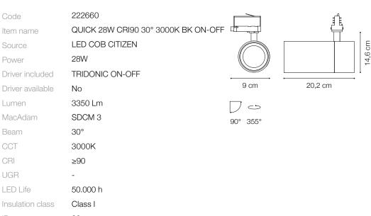
LED Life 50.000 h Insulation class Class I IP 20 Material Aluminum Warranty 5 years Net Weight 1,120 Kg Volume 0,0061 m<sup>3</sup>
